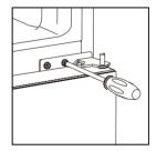
Laying down the refrigerator, take out the adjusting feet as below, then unscrew the lower hinge by cross screwdriver.
