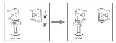
6. Refit the bracket fitting the bottom hinge pin. Replace both adjustable feet. Transfer the lower door to the property position.
